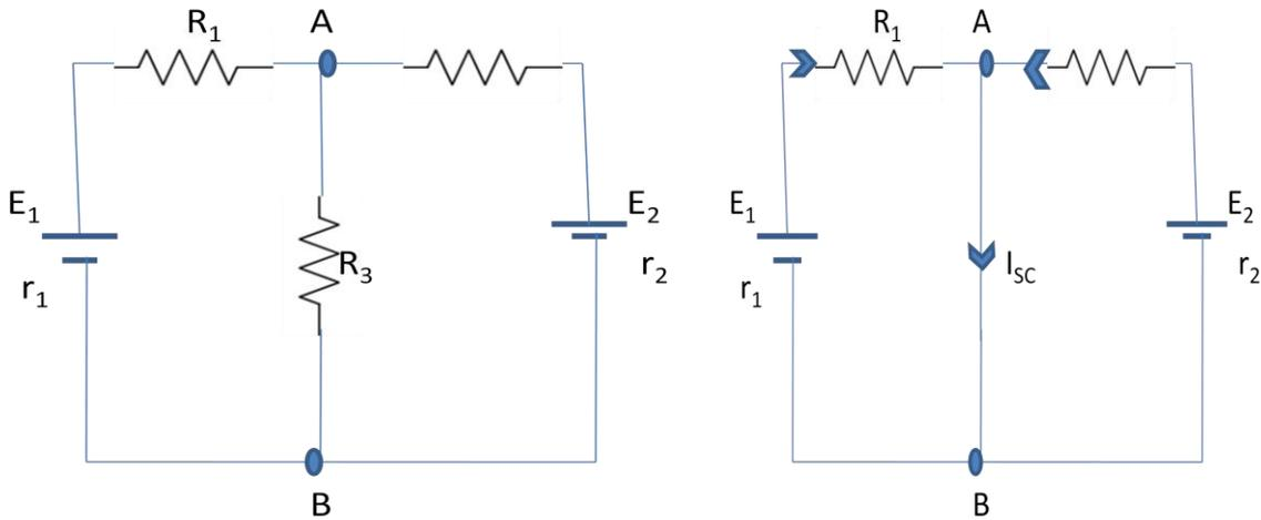
$$I_{SC} = \frac{E_1}{R_1} + \frac{E_2}{R_2} = E_1 G_1 + E_2 G_2$$
