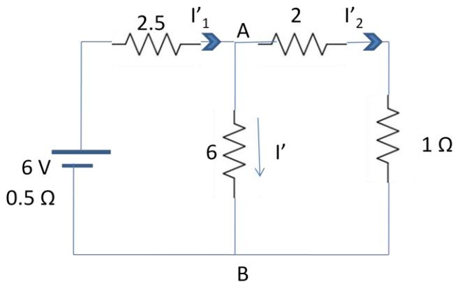
Here only 6 V is considering by removing 12 V with its internal resistance of 1 Ω.
