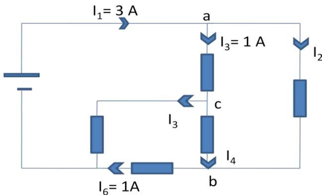
**Solution:** At junction a,  $I_1$  is entering and  $I_2$ ,  $I_3$  are leaving. So according to KCL:
