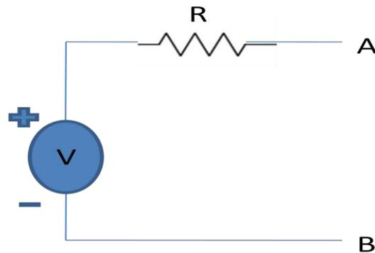
**Fig.16(a)** Voltage source with series resistance
