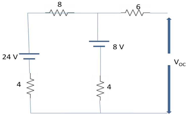
For finding  $V_{OC}$ , net voltage =  $24 - 8 = 16 \text{ V}$
