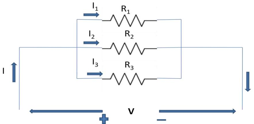
Fig 7 parallel connection of resistances
