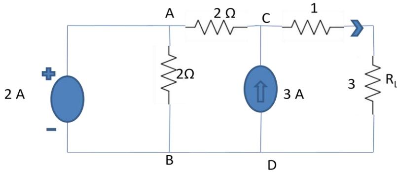
Now, the 2A current source with parallel resistance  $2\ \Omega$  can be converted into equivalent  $4\text{V}$  voltage source with  $2\ \Omega$  series resistance. Again, the series connection of two  $2\ \Omega$  resistance can be converted into one  $4\ \Omega$  resistance.
