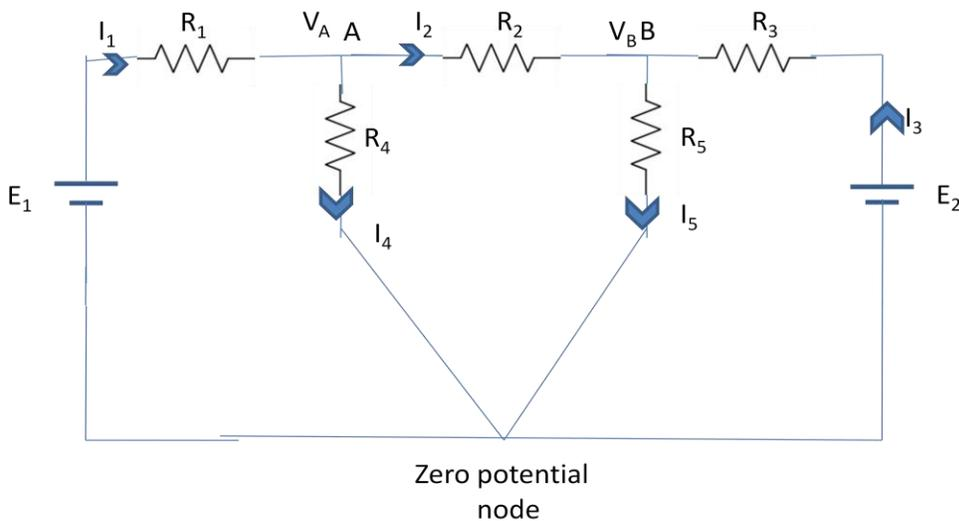
**Fig.21** Node voltage Analysis
