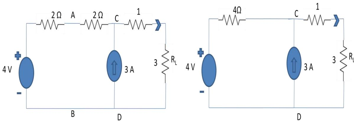
In the above figure, you can see that there is a series connection of  $4\text{V}$  voltage source and  $4\ \Omega$  resistance. So, it can be converted into equivalent current source of  $1\text{A}$  with parallel resistance of  $1\ \Omega$ .
