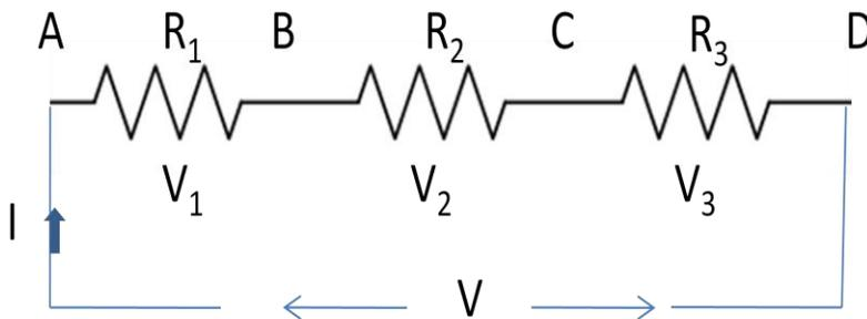
**Fig 6** Series connection of resistances
