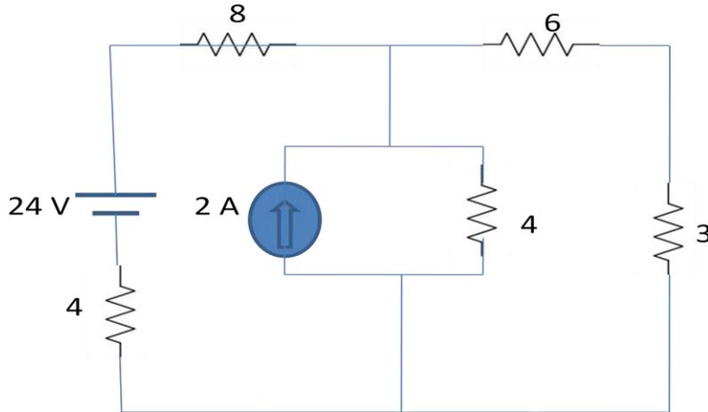
**Solution:** First of all we have to convert 2 A current source and parallel resistance to a voltage source with series resistance by source conversion technique and redraw the circuit.
