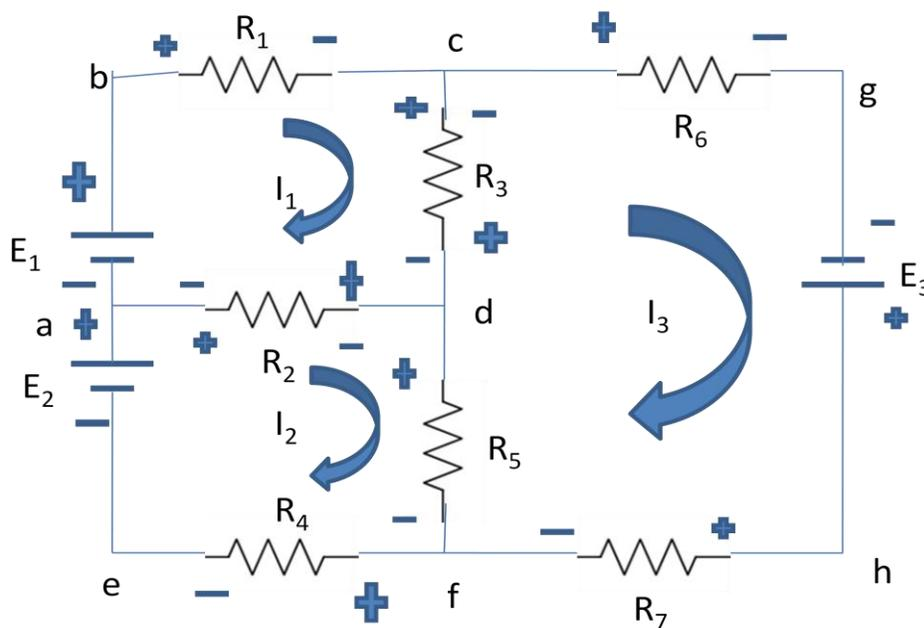
**Fig.20** Mesh analysis of a circuit
