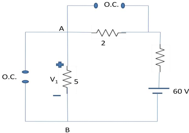
$V_1 = 60 \times \frac{5}{5+2+3} = 30 \text{ V}$  ; its value is taken positive, because current through the  $5 \Omega$  resistor from A to B, so making the upper end of resistor positive and the lower end negative.
