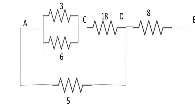
**Solution:** Resistance between A and C =  $6 \parallel 3 = \frac{6 \times 3}{6 + 3} = 2\Omega$
