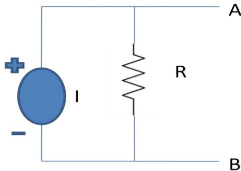
**Fig.16(c)** Current source with parallel resistance
