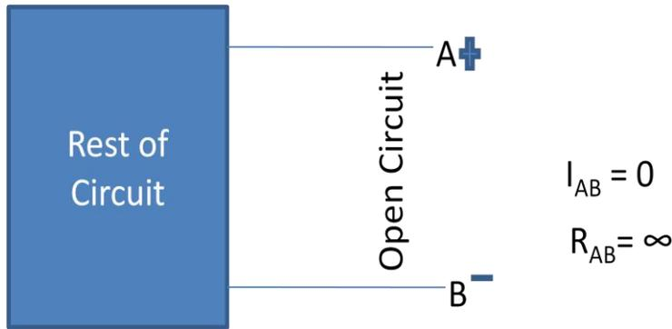
**Fig.11 Open circuit**
