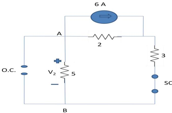
In the above figure, the 6 A current source has two parallel circuit across it; one having the resistor of  $2\Omega$  and other path having the series connection of resistances  $(3+5) = 8 \Omega$ . Using the current divider rule, the current through  $5 \Omega$  resistor=
