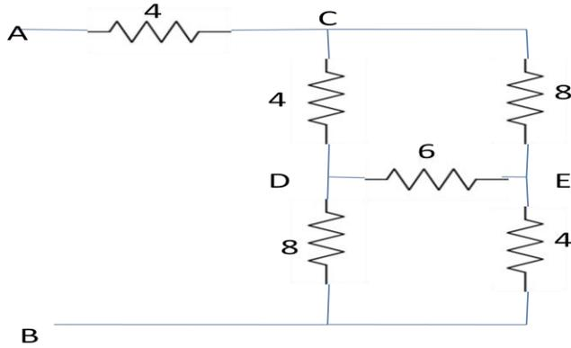
**Solution:** For finding out  $R_{AB}$ , we have to convert the delta CDE into its equivalent star. So,
