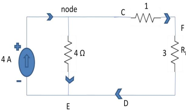
So, 4A current is divided into two equal parts at node because each of the two parallel paths has a resistance of  $4\ \Omega$ .  $I_{RL} = 2\ \text{A}$ .
