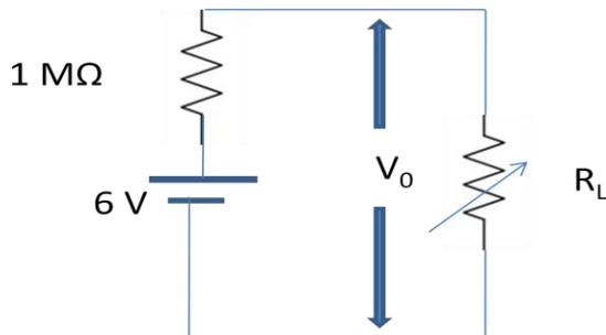
6 V battery has an internal resistance of  $1 \text{ M}\Omega$  and load resistance varies between  $20 \text{ K}\Omega$  to  $200 \text{ K}\Omega$ . So, current supplied by the source varies from  $6/1.02 = 5.9 \mu\text{A}$  to  $6/1.2 = 5 \mu\text{A}$ . So, it is seen that even when load resistance increases 10 times, current decreases by  $0.9 \mu\text{A}$ . Hence source can be considered constant current source.
