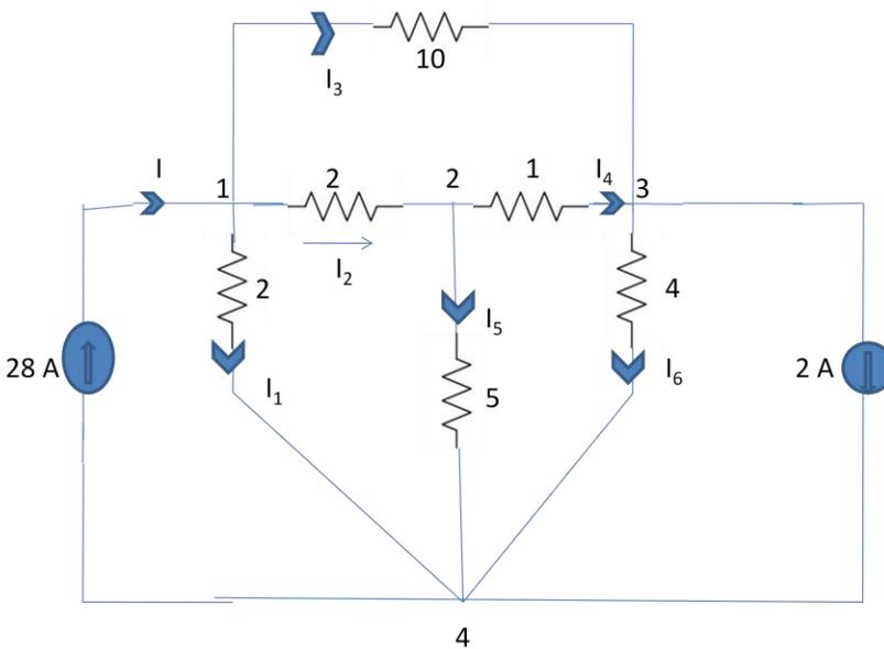
**Solution:** Node 1:  $V_1 \left( \frac{1}{2} + \frac{1}{2} + \frac{1}{10} \right) - \frac{V_2}{2} - \frac{V_3}{10} = 8$
