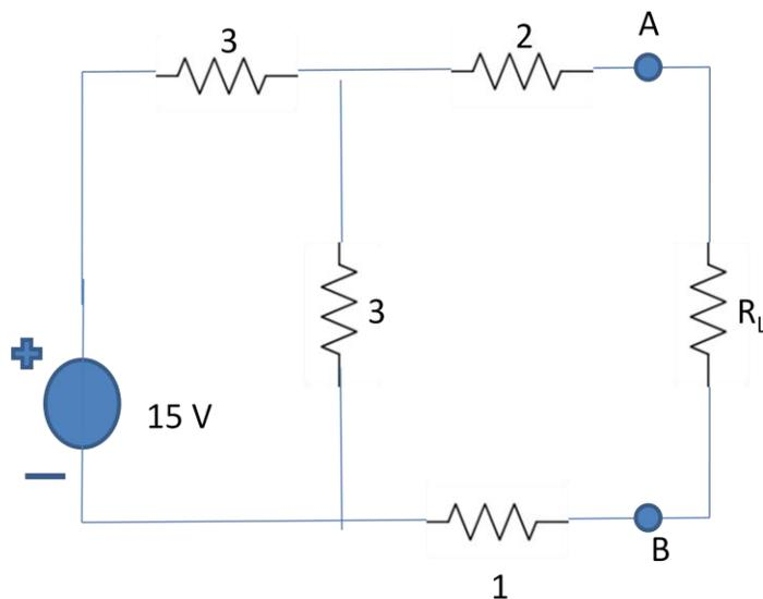
**Solution:** First remove  $R_L$  to find the equivalent Thevenin's source of the circuit to the left of terminals A and B.
