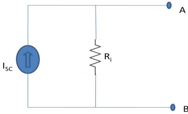
**Fig.25** Norton equivalent circuit
