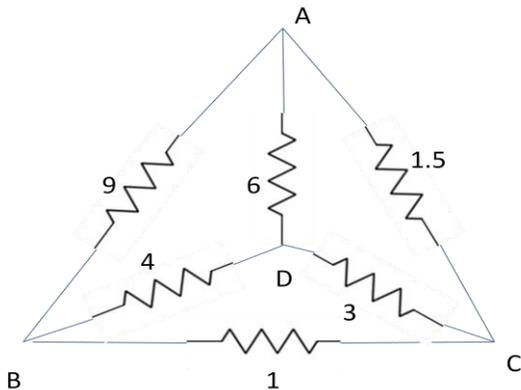
**Solution:** There are two combinations of resistances in above figure i.e. inner star and outer delta. So, the inner star can be converted into equivalent delta and combined in parallel with the outer delta ABC.
