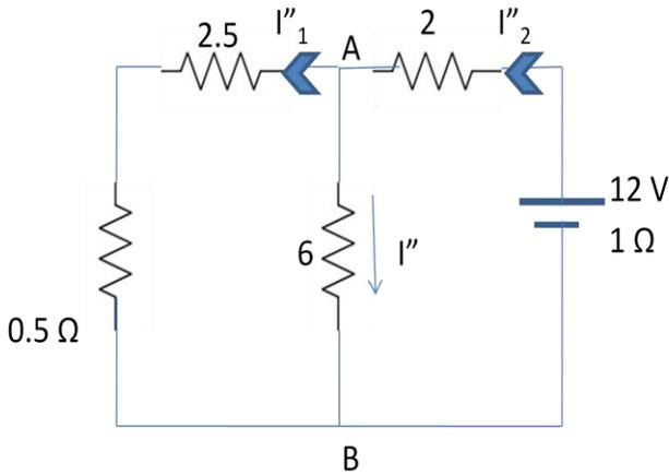
Here only 12 V is considering by removing 6 V battery with its internal resistance of  $0.5 \Omega$ .
