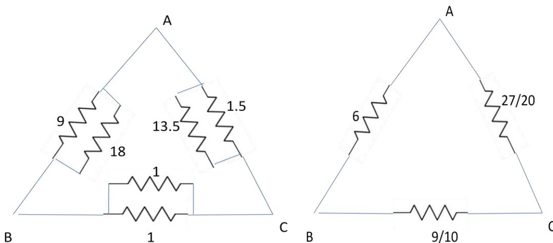
$R_{AB}$  is the resistance between terminals A and B means  $6 \parallel (27/20 + 9/10)$ ,  $R_{BC}$  is the resistance between terminals B and C i.e.  $9/10 \parallel (6 + 27/20)$  and  $R_{CA}$  is the resistance between terminals C and A i.e.,  $27/20 \parallel (6 + 9/10)$ .
