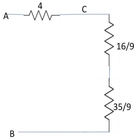
The two parallel path between S and B can be reduced to a single resistance of  $35/9$  i.e.,  $(12/9 + 8) \parallel (24/9 + 4)$ .
