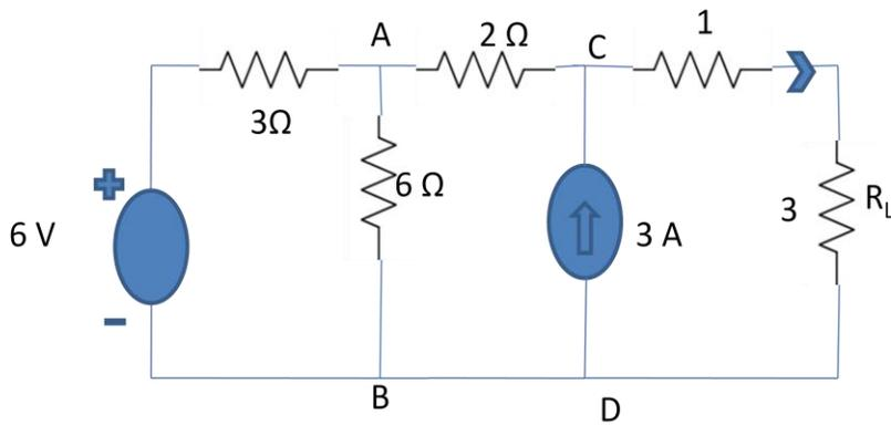
**Solution:** As shown in above figure, 6 V voltage source with a series resistance of  $3\ \Omega$  has been converted into 2 A current source with  $3\ \Omega$  resistance in parallel. By redrawing the circuit again,
