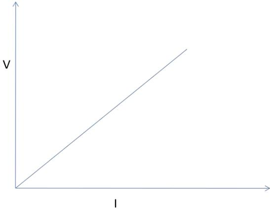
**Fig.5** The V-I characteristic of resistance
