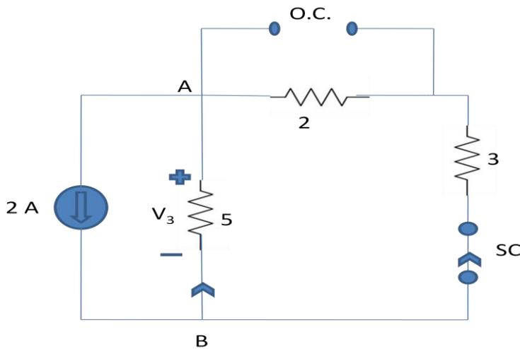
Current 2 A divides equally at point B, because the two parallel paths have equal resistance of  $5 \Omega$  each.
