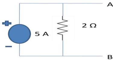
**Solution:** The open-circuit voltage across terminals A and B in above figure is,
