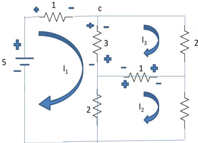
**Solution:** In mesh-1, mesh equation is  $6I_1 - 2I_2 - 3I_3 = 5$
