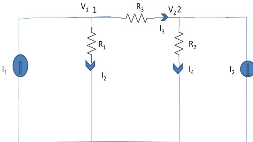
**Fig.23** Node Voltage Analysis with Current Sources
