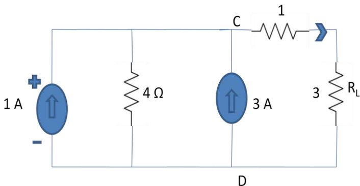
Here, there are two current sources 1A and 3A entering into a node and leaving through CE and CFD path like below, then we can apply KCL here to find out current through  $R_L$ . So,
